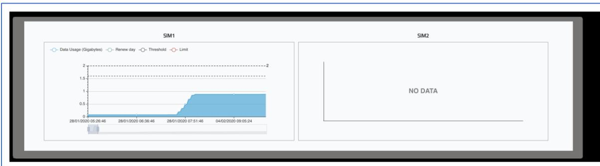
The SIM STATS shows the amount of data transfer with a cellular modem connection for a specified time period. Data is separated by each installed SIM card in that cellular modem. Data is split between data transmitted (TX) and data received (RX).
