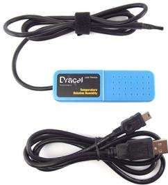
Acquire environmental temperature and relative humidity readings. Easily integrate the compact probe in space-constrained locations, and get precise measurements from the factory-calibrated, linearized, and temperature-compensated digital sensor chip. The built-in particle filter protects the components against dust, soot, and other particle contaminants. Control and read status using CLI, Web, SNMP or Restful APIs.
